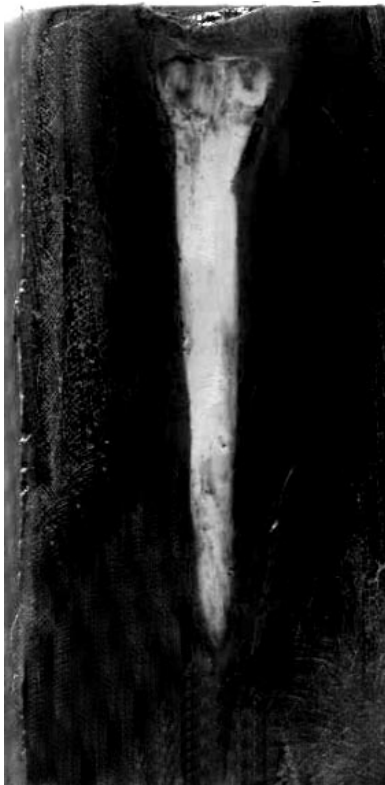
FIG. 4. Cross section of the lead sample with h_0 \approx 9 cm, R \approx 2.2 cm. Note that the pipe is closed from the top, forming a cavity.
