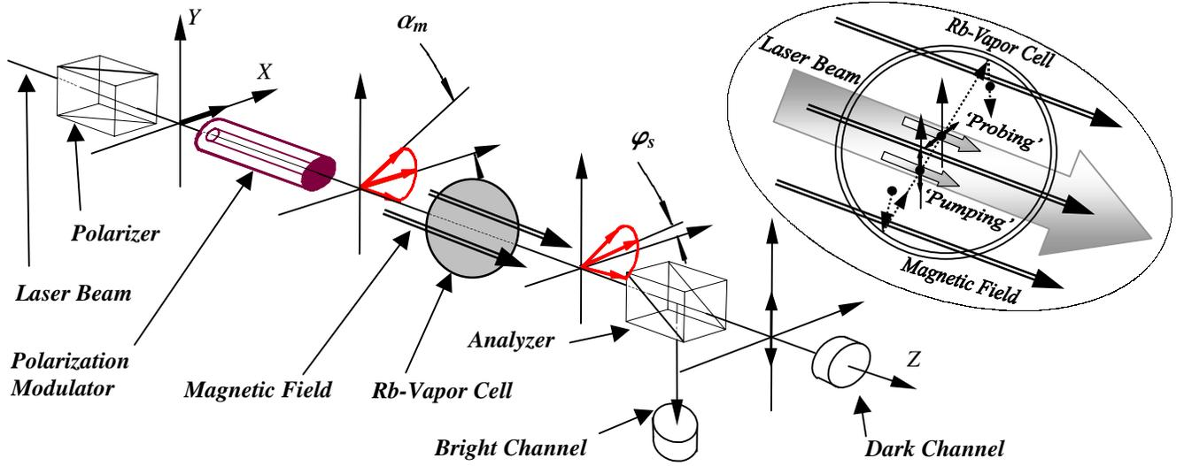
**FIGURE 1.** Schematic of an experiment to observe NMOE with Rb vapor. The Rb atoms aligned by linearly polarized light represent a magneto-optically active medium in a magnetic field. The measure of the polarization rotation angle is the intensity of light passing through the analyzer crossed with the polarizer. The details of the modulation polarimeter are described in the text. The inset illustrates the mechanisms for the coherence effect.
