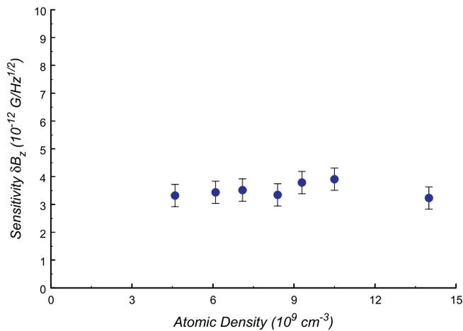
FIG. 8. Shot-noise-limited sensitivity as a function of atomic density for the  $F_g = 3$  component of the D2 line, light intensity = 20 mW/cm<sup>2</sup>. Light frequency at each point is chosen to achieve optimum sensitivity.
