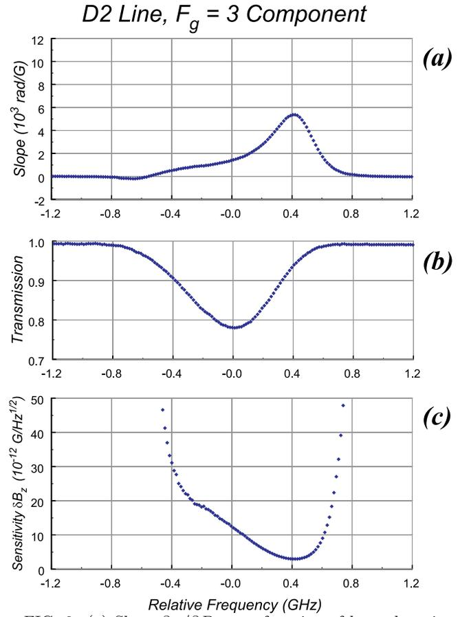
FIG. 6. (a) Slope  $\partial\varphi/\partial B_z$  as a function of laser detuning for the  $F_g = 3$  component of the Rb D2 line (laser intensity  $\approx 4.5$  mW/cm<sup>2</sup>); (b) Normalized light transmission; (c) estimated shot-noise-limited sensitivity  $\delta B_z$ .
