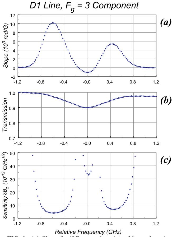
FIG. 5. (a) Slope  $\partial\varphi/\partial B_z$  as a function of laser detuning for the  $F_g = 3$  component of the Rb D1 line (laser intensity  $\approx 1$  mW/cm<sup>2</sup>); (b) Normalized light transmission; (c) estimated shot-noise-limited sensitivity  $\delta B_z$ .
