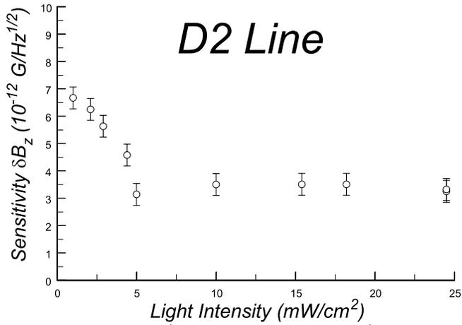
FIG. 7. Optimum (with respect to frequency) shot-noise-limited sensitivity as a function of light intensity for the  $F_g = 3$  components of the D1 and D2 lines. Data taken at room temperature (20 °C, atomic density  $\approx 4.5 \times 10^9 \text{ cm}^{-3}$ ). Note that the scale of the horizontal axis is five times larger for the D2 line.
