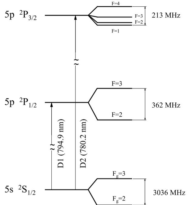
FIG. 1. Partial energy level diagram of  $^{85}\text{Rb}$  (nuclear spin =  $5/2$ ) with hyperfine splittings and relevant transitions (not to scale).
