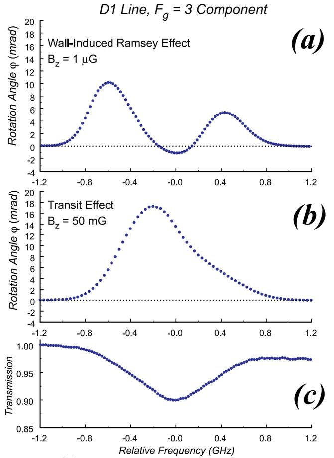
FIG. 4. (a) Wall-induced Ramsey rotation spectrum, light intensity is  $1.2 \text{ mW/cm}^2$ , beam diameter  $\approx 3 \text{ mm}$ . (b) Transit effect rotation spectrum, light intensity is  $0.6 \text{ mW/cm}^2$ . (c) Light transmission spectrum for light intensity =  $1.2 \text{ mW/cm}^2$ . Overall slope in light transmission is due to change in incident laser power during the frequency scan.
