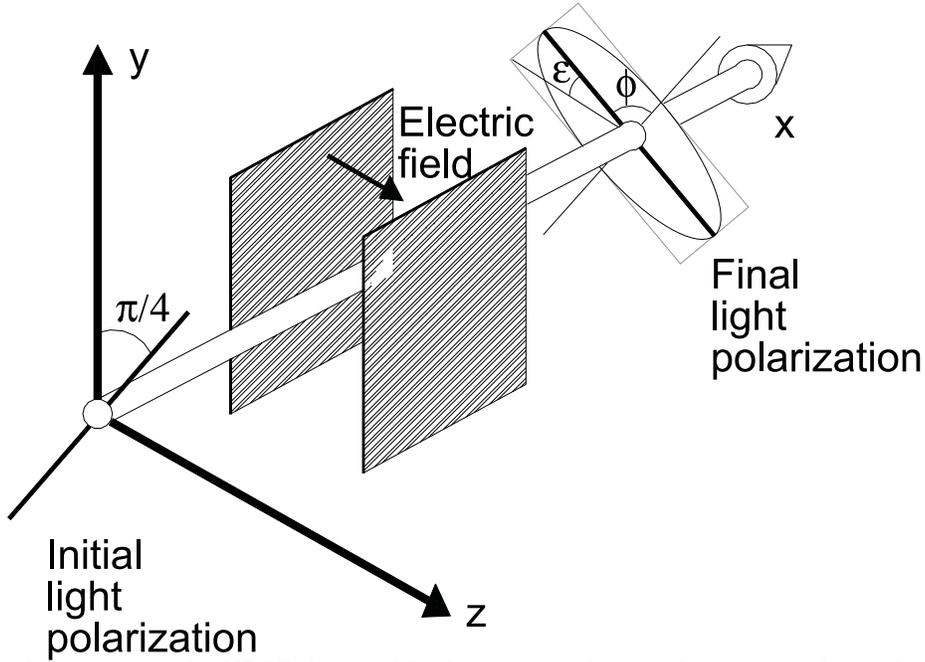
FIG. 1. Geometrical arrangement for NEOE discussed in the text. Angles  $\phi$  and  $\epsilon$  correspond to polarization rotation and ellipticity, respectively.
