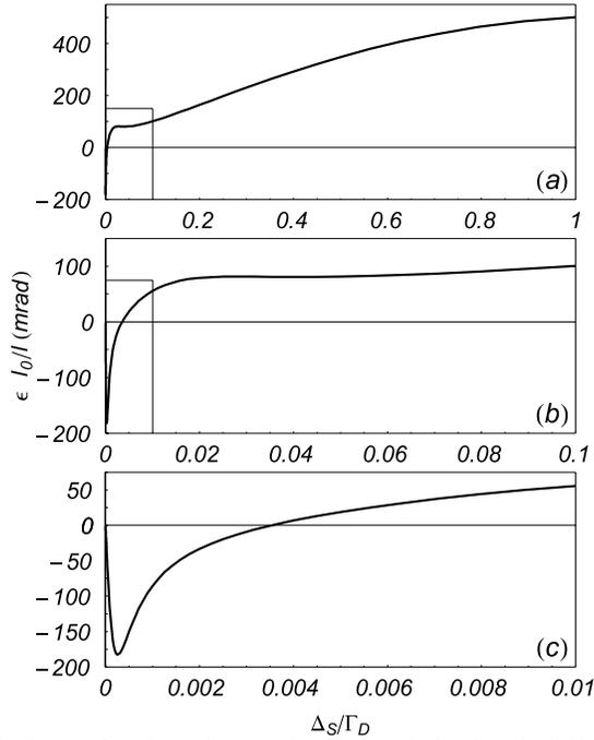
FIG. 4. Ellipticity per unsaturated absorption length as a function of the Stark shift normalized to the Doppler width. *a*: linear effect; *b*: Bennett structure effect; *c*: coherence effect. The light frequency is tuned to the electric field-free resonance. Various parameters used in the calculation are discussed in the text.
