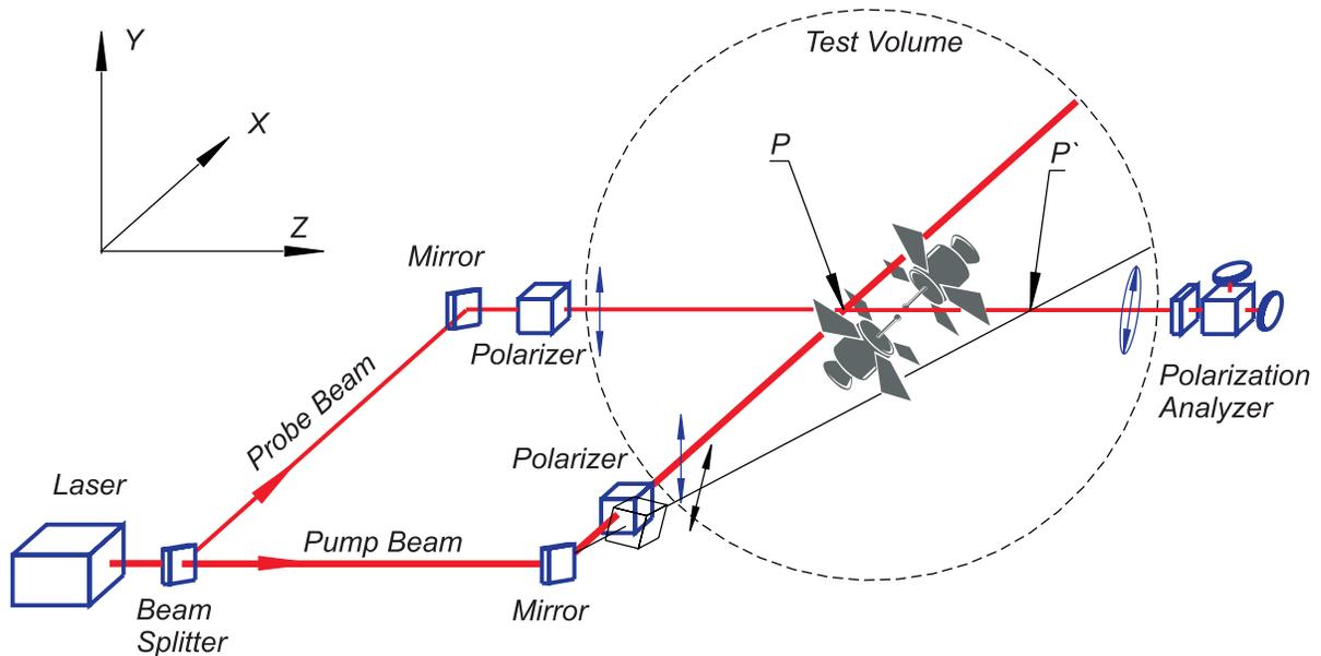
FIG. 5. Schematic for electromagnetic field measurement.
