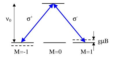
Fig. 1. An F=1  $\rightarrow$  F'=0 atomic transition. In the presence of a longitudinal magnetic field, the Zeeman sublevels of the ground state are shifted in energy by gµB·M. This leads to a difference in resonance frequencies for right- and left-circularly polarized light ( $\sigma^{\pm}$ ).
