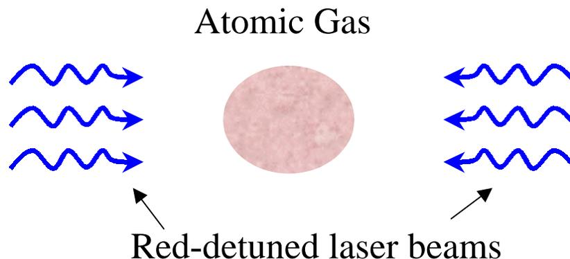
**3-D:** Multiply this by 3 (i.e. shine pairs of beams in three orthogonal directions).
